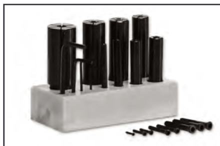
Figure 11.3 Hardened steel mandrels have a slight ground taper and expanding collar.
