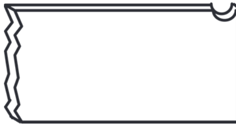
Figure 9.7 A crater starts the chip curling smoothly.
