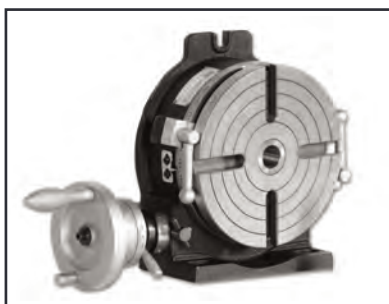
Figure 9.3 Rotary tables let you cut gears, precision holes, and curved slots.
