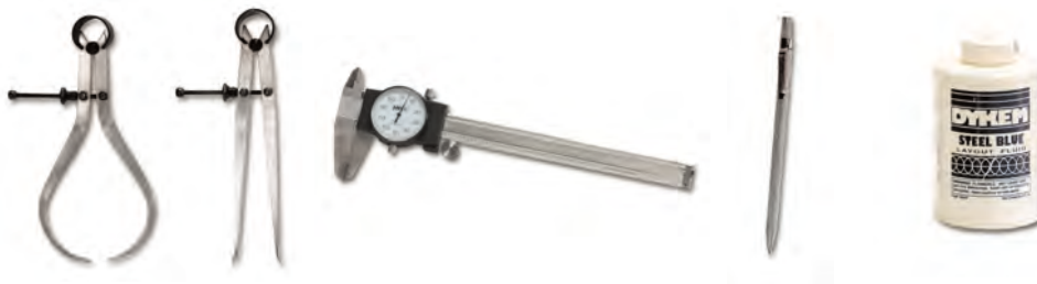
Figure 11.3 Use centering instruments include calipers and dividers.
