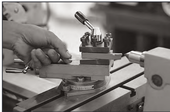
Figure 10.1. Placing shims under the tool can correct cutting tool height.
