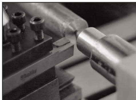
Figure 3.2 With a half-center you can extend the tool across the entire face of the work.
