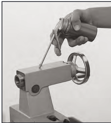
Figure 6.8 Oil the two buttons on the top of the tailstock.
