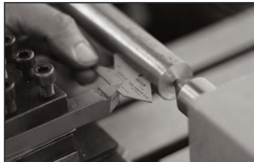
Figure 6.6 Use a center or thread gauge to correct cutter alignment error when squaring the cutter with the workpiece.
