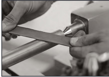
Figure 2.4 With a file, take full strokes at an oblique angle and never hold the file still.
