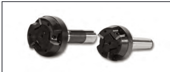
Figure 23.2 Inserted tooth face milling cutters face mill large surfaces.
